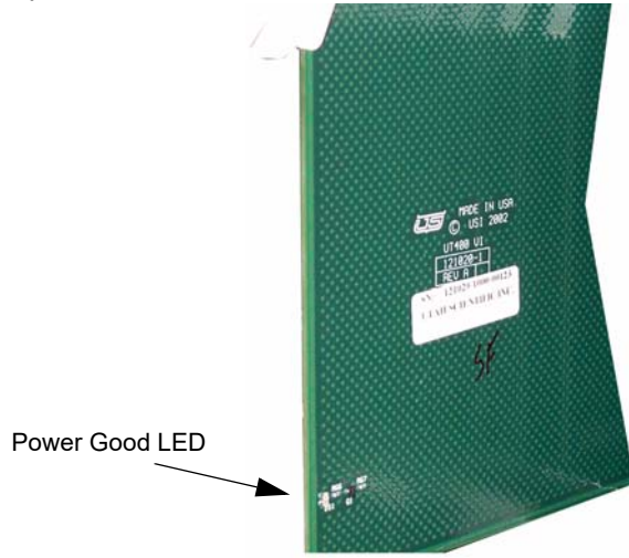
FIGURE 4-4. Power Good LED
