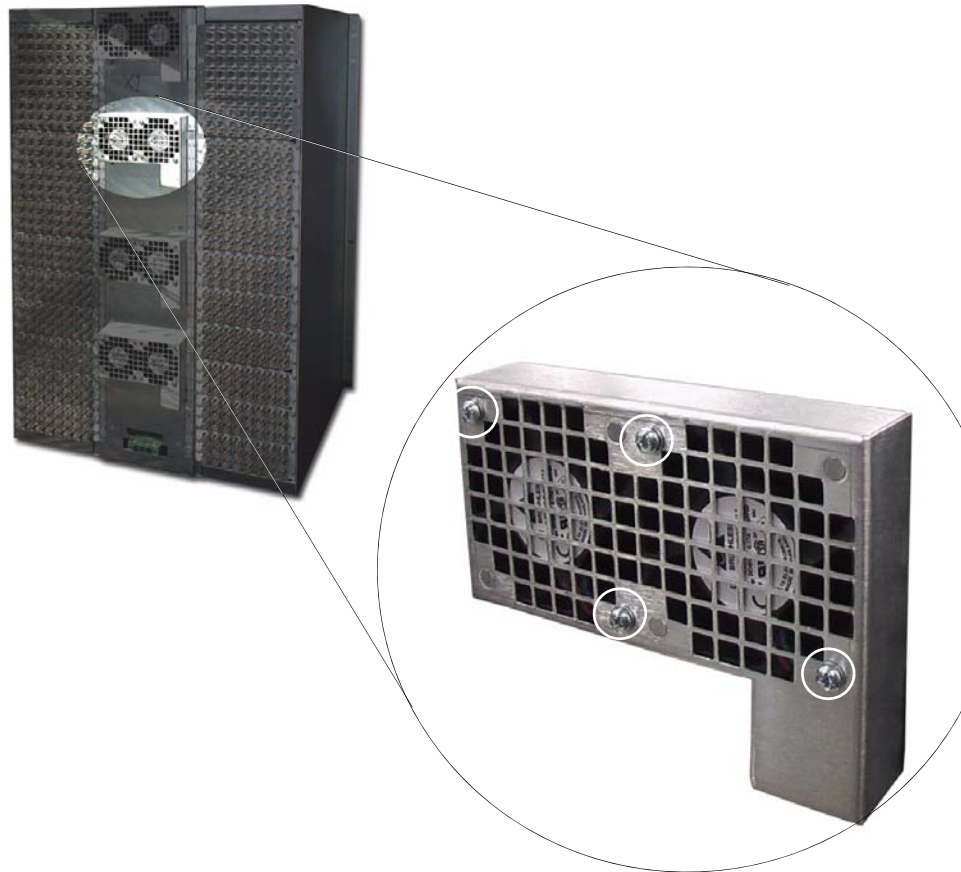
FIGURE 3-7. Fan location and removal
