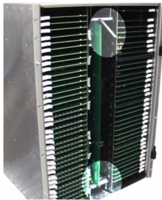
FIGURE 3-6. Crosspoint Board Replacement and Removal
