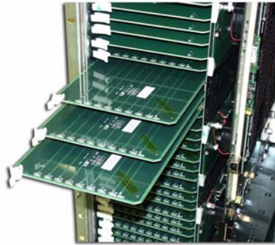
FIGURE 3-5. Input/Output Board Replacement and Removal
